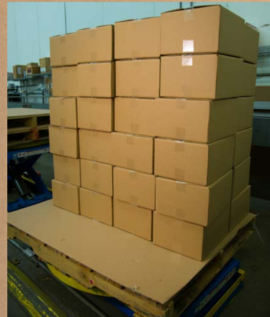
The 35 F to 40 F temperatures of the facility can impact the reliability of case seals, so Kent Quality Foods uses a packaging tape that’s specifically designed for colder environments.
