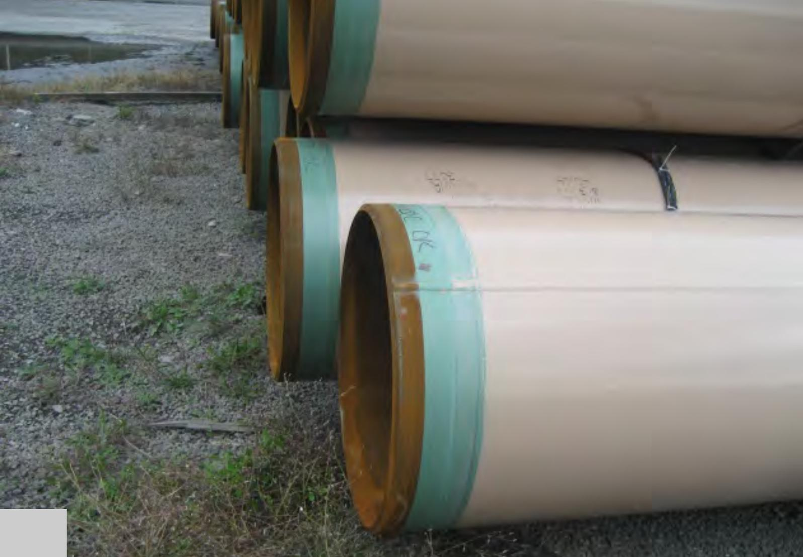
*Pipe ends must remain free of protective coating to ensure they can be welded in the field.*
